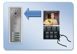
If there isn't any active call, with the camerabutton the spy-function can be enabled and disabled. If the spy-function is activated, the video window shows all the video sources defined for the external unit selected as doorspy. With the appropriate horizontal swipe gesture on the active video window it's possible to switch between the single video sources.
