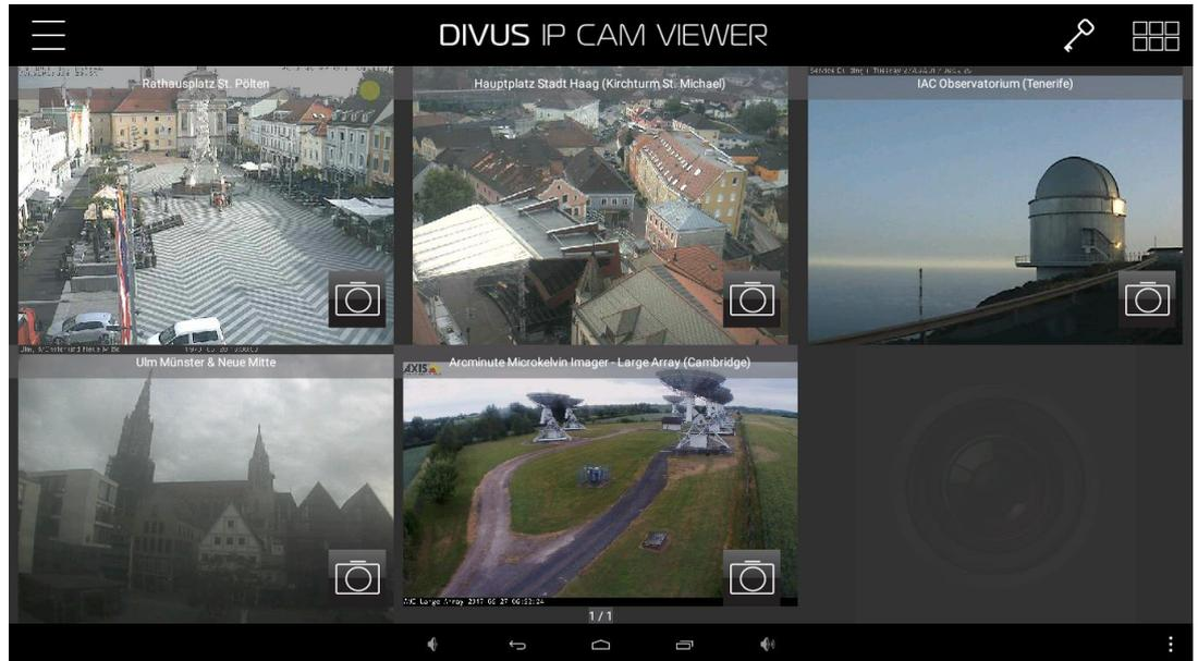
Each configured camera has its own frame, and depending on the layout and orientation they are distributed differently. On bottom in the middle is the page indicator, the first number shows the current page, the second number shows the total number of pages. Depending on the amount of cameras and selected layout the page count may change. It's possible to switch to the next/previous page with a horizontal swipe on the main screen.
