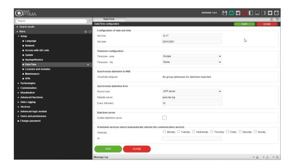
Note: The D+ does not have a battery for storing the date and time. Therefore a power loss might cause it to loose its correct date/time settings.
