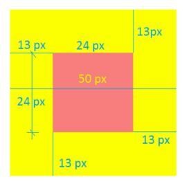
The dimensions are 50x50 pixel externally. In order to be published correctly with both normal and small icons (see chapter 4.4.4), the graphical content should occupy only the inner, red area measuring 24x24 pixel.
