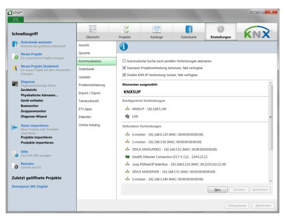
Click on "New" to open the pop-up "New connection"; enter a name for the connection, specify "KNXNet/IP" as the type and manually enter the IP of the server and define "3671" as the port (do NOT activate NAT mode!).
