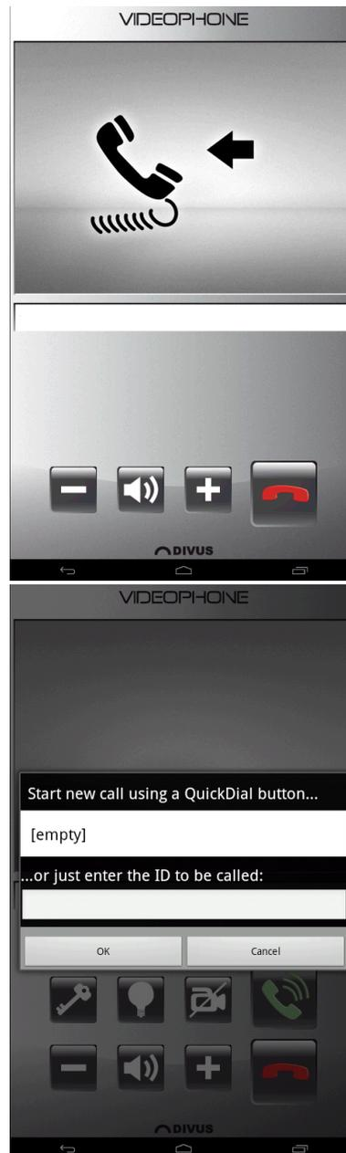
Even when the **DIVUS VIDEOPHONE** app is closed, it must be reachable for incoming calls and open its interface automatically. In order to realize this, the **VIDEOPHONE** app uses a background service that handles the registration on the VoIP server and manages incoming calls.
